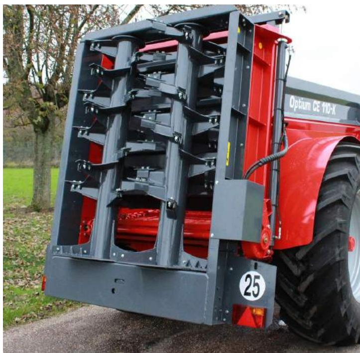
The Optium range of Manure Spreaders feature the unique Perard Double Helix Rotor System which is proven to deliver an unrivalled quality of spread in the field.
